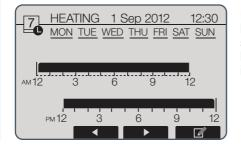
Hours of the day are shown as a bar across the main part of the screen. Where the bar is solid black, heating/DHW (whichever is selected) is allowed.
