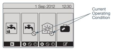
Turning on Priority Hot Water / Hot Water / Heating Forced domestic hot water: To activate press F1 Domestic hot water operating mode: To change mode press F2 Space heating operating mode: To change mode press F3 Holiday mode: To access Holiday screen press F4
